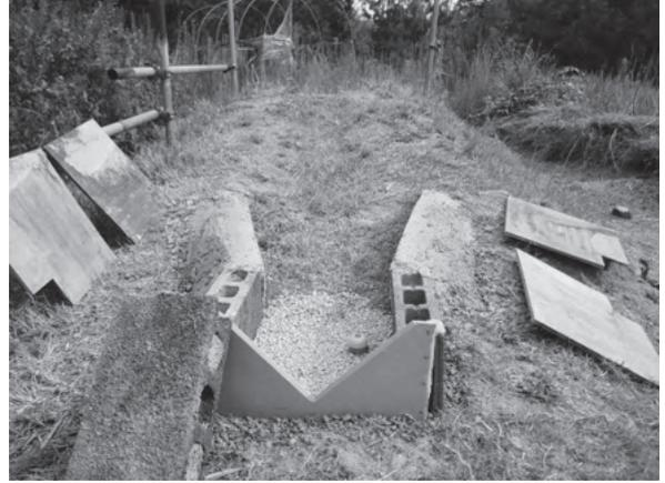
Fig.1: MCRWH system developed at the experimental field of Kyoto University in Maizuru
